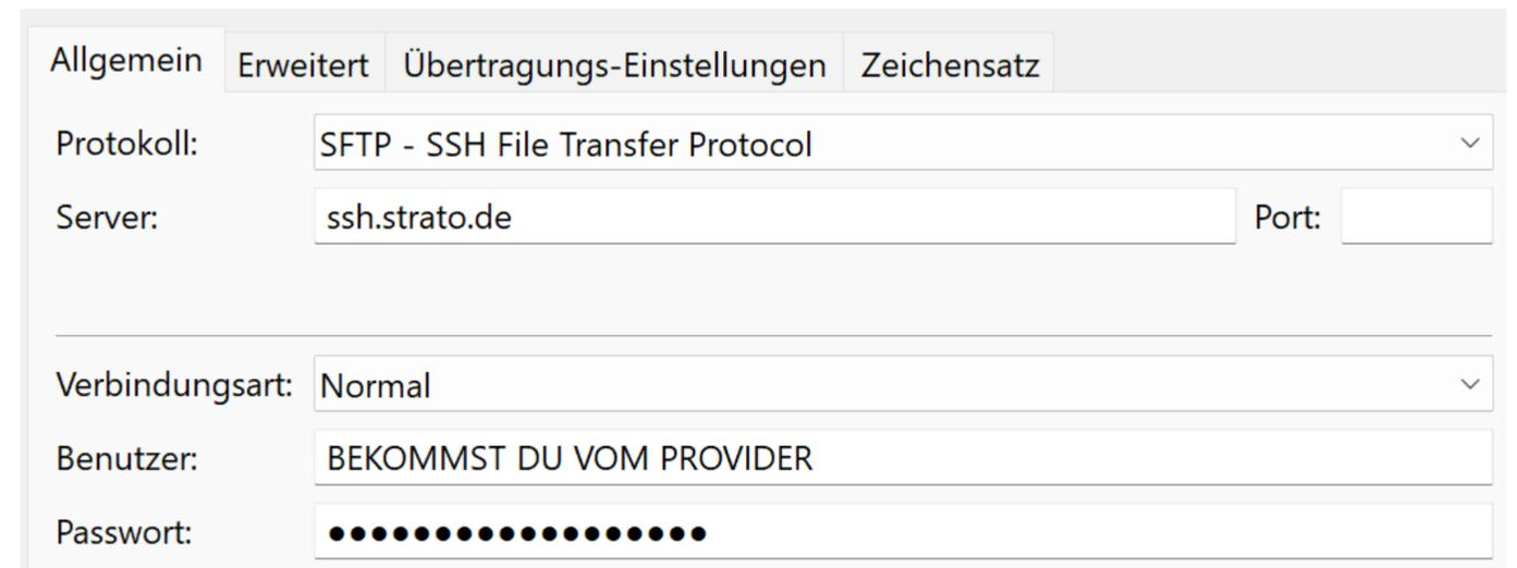
The screenshot shows the FileZilla connection settings dialog box. The 'Allgemein' tab is selected. The 'Protokoll' dropdown is set to 'SFTP - SSH File Transfer Protocol'. The 'Server' field contains 'ssh.strato.de' and the 'Port' field is empty. The 'Verbindungsart' dropdown is set to 'Normal'. The 'Benutzer' field contains 'BEKOMMST DU VOM PROVIDER' and the 'Passwort' field is masked with dots.
